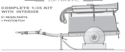
The CO2 Löschgerät auf Anhängerfahrgestell A1 - CO2 fire extinguisher on trailer chassis A1 - was used by the Luftwaffe units to fight fires of the aircrafts, electrical installations, and other devices, were water and foam was not an option.
